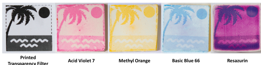
Figure 2. Photographs demonstrating the color change of each ink upon UVA irradiation ( I_0 = 3.26 \text{ mW cm}^{-2} ) through a printed transparency film, on STOClimasan Color paint. Both AV7 and MO were irradiated for 30 min, whereas BB66 and Rz were irradiated for approximately 0.1 min.
